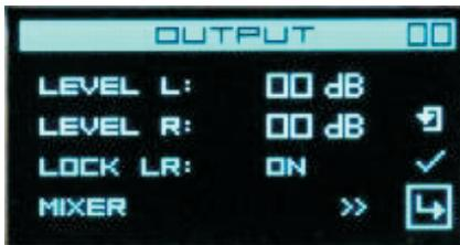
The channels' output level is adjusted here. Like the input attenuator menu, **LOCK LR** parameter combines the volume level control for both channels.
