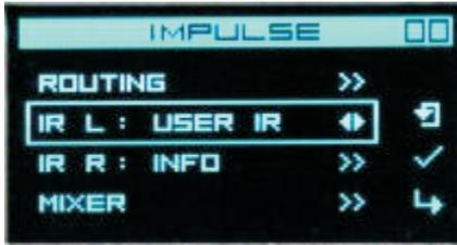
**USER IR** – this is the main menu to choose the impulse. All the user impulses should be saved to a /IR folder located in the root directory of the SD card. Impulses should be 24 bit 48 kHz WAVE PCM1 format. IRon Cab can display up to 1000 impulses. Subfolders not supported.
