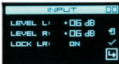
**INPUT LEVEL** menu is used to set up the input attenuator.
