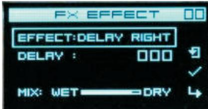
**DelayR** – right channel signal delay, used for a pseudo-double tracking effect. The values are in samples. Most audibly noticeable when set to 20,
