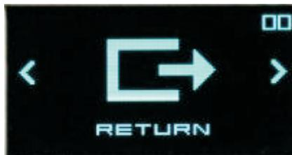
Swiping between the menu items is done by turning the encoder left or right. TO enter a desired menu item press the encoder.
