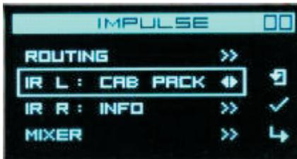
**CAB PACK** – is the mode for loading the CAB files. A CAB file is a user library of impulses. They are used to arrange the impulses for convenient use. It is essential when using commercial (paid) packs. Navigation is understandable, convenient and quick. You can create your own CAB files using special PC software. CAB file
