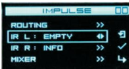
**EMPTY** – if an impulse is not loaded into the preset, this menu item displays EMPTY. If the impulse is loaded, once the EMPTY option is chosen – the Bypass mode will be loaded.
