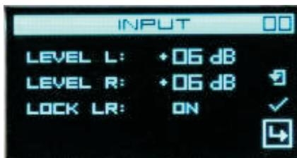
**INPUT LEVEL** menu is used to set up the input attenuator.
