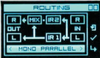
**MONO PARALLEL** – in this mode the signal is taken from the left input (L), but two impulses can be assigned in parallel. Depending on the mixer settings, you can route a processed, a non-processed or a signal mix to right output (R).
