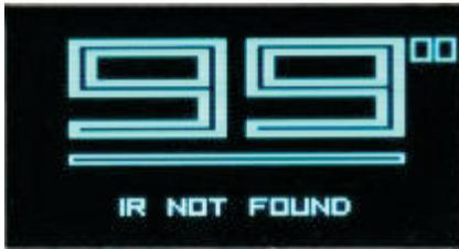
If the preset is empty (Impulse not assigned), then the preset number is written with an empty font. The encoder is used to swipe between the presets and the number of an actual preset is displayed in the upper right of the screen. Press the encoder to choose the needed preset.
