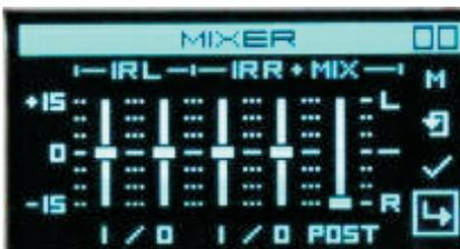
This menu is used to set the input and output signal levels for each impulse and the channels balance using the MIX fader. Depending on the routing scheme, an input signal can be mixed to the after-impulse signal, the signals processed with different impulses can be mixed, or channels can be mixed as well.
