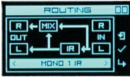
**MONO 1 IR** – signal is taken from the left input (L) and only one impulse can be assigned to it. It is a basic default setup and a particular case of MONO SERIAL setup. This is designed not to set up two impulses if only one is going to be used. In this case IR on Cab works in pure mono mode. Depending on the mixer settings, you can route either a processed or a non-processed signal to right output (R). It can be rather useful, in case of bass guitar, for instance.
