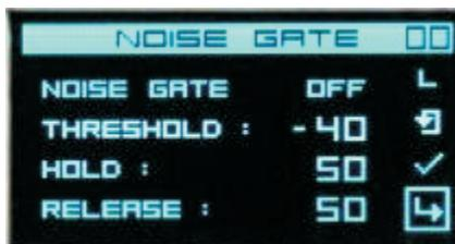
**NOISE GATE:** ON/OFF activates/deactivates the noise gate
