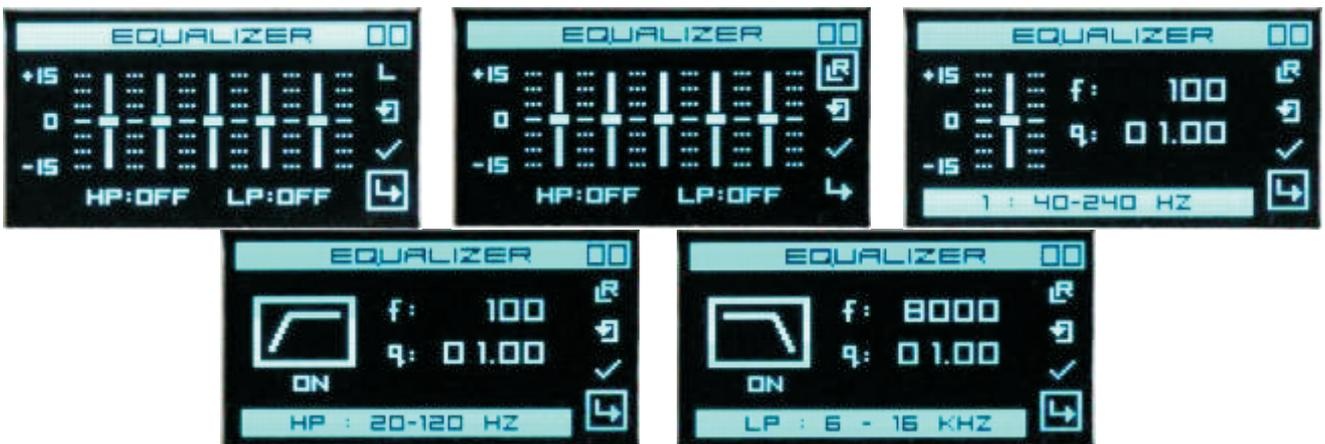
The parameters can be set by choosing a needed fader or a button. The EQ can be adjusted either separately for each channel or simultaneously for both by choosing L+R mode in the upper right of the screen.
