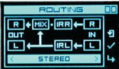
**STEREO** - in this mode the signal is taken both from the left input (L) and right input (R). You can choose a separate impulse for each channel. This mode allows one musician to play in a stereo mode or two musicians using their own FX chains separately.
