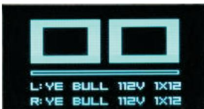
If a preset is not empty (a preset(s) assigned), then the preset number is displayed in bold, and you can see the preset's name below. Depending on the routing scheme, one or two impulse names can be displayed.
