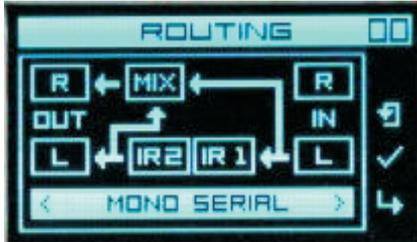
**MONO SERIAL** – in this mode the signal is taken from the left input (L), but two impulses can be assigned in serial (e.g. Impedance Curve Impulse and Cabinet Impulse). Depending on the mixer settings, you can route either a processed or a non-processed signal to right output (R).
